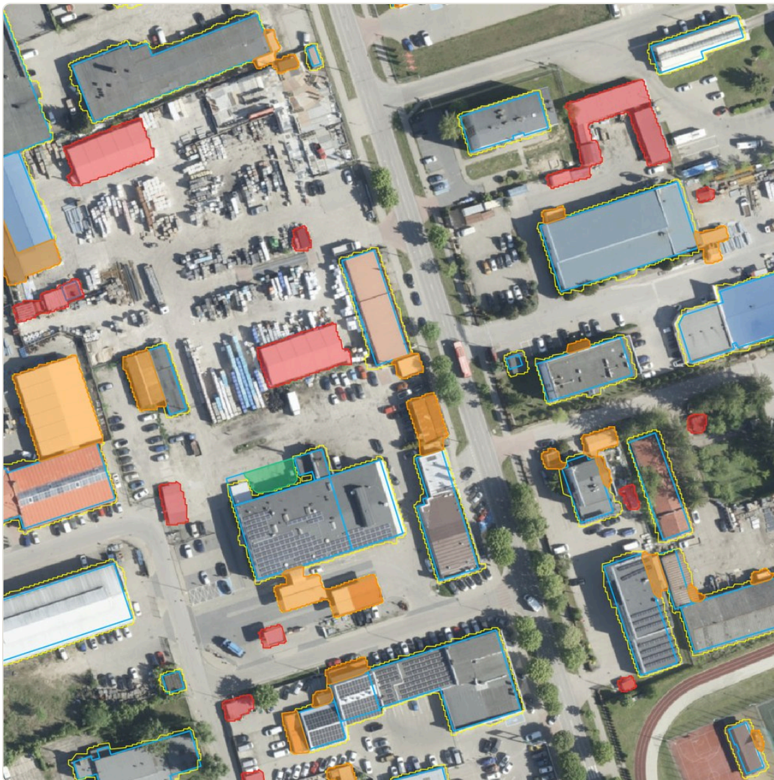
Figure 1. EtK, 250 × 250 m extract. Blue: EGiB buildings (aggregated WFS service, as of 3 October 2026). Yellow: outlines from LiDAR 2025 (script 1). Red: NOWY. Orange: ROZBUDOWA. Green: ZMNIEJSZENIE. Background: GUGiK orthophotomap (WMS). Figure from the first trial (script 1 before the correction of 4 October 2026, outlines about 0,5 m wider).
